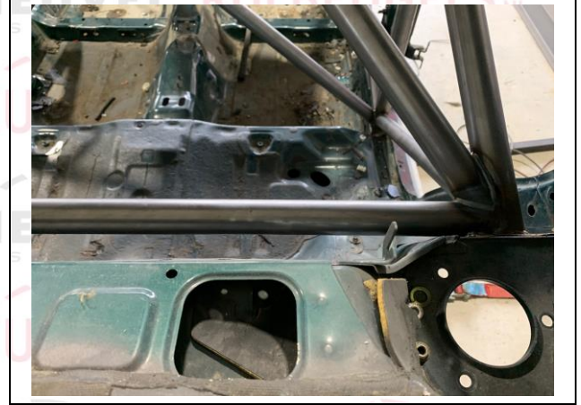
PHOTO 13 SHOULDER HARNESS ATTACHMENT - CO DRIVER
