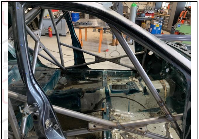
PHOTO 11 ANTI-INTRUSION DOORBAR - CO-DRIVER
