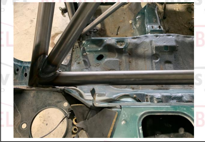
PHOTO 12 SHOULDER HARNESS ATTACHMENT - DRIVER
